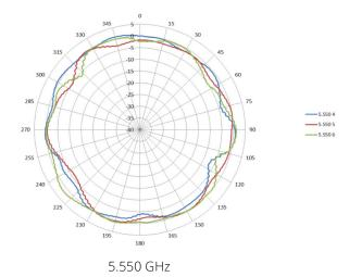
Horizontal or azimuth plane (top view, 30 degrees downtilt)
