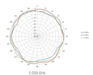
Elevation plane (side view, 0 degrees angle)
