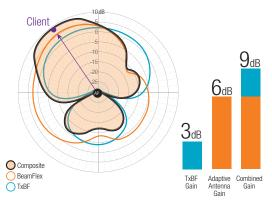
Ruckus access points uniquely combine the benefits of adaptive antenna arrays with transmit beamforming to provide unmatched reliability and TCP performance in real-world deployments
